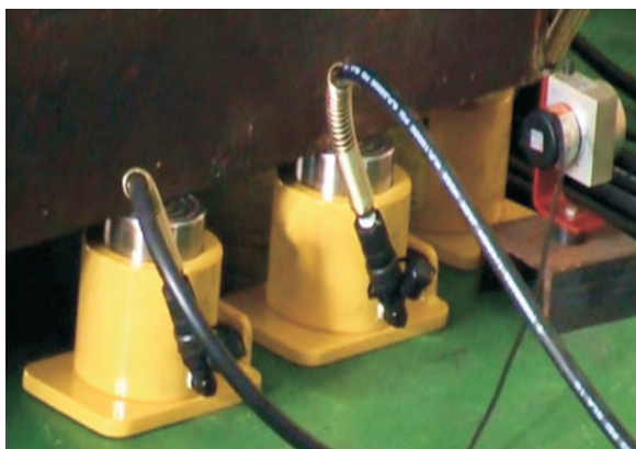
RCS-502 捷运系统同步实例应用 RCS-502 Rapid transit system Synchronous Lift application
